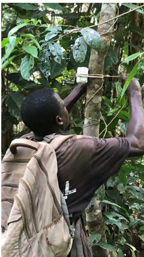
Left: Andrew Gweh, a research student from the University of Liberia setting up Audiomoth, a bioacoustic recording device that records vocalising animals. Using specialised software, the activity of bird and bat species can be quantified from the Audiomoth recordings.
